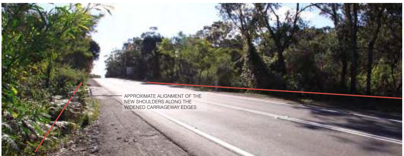
Figure 4.2.4: Existing view looking west along Mona Vale Road within Landscape Character Zone 3.
