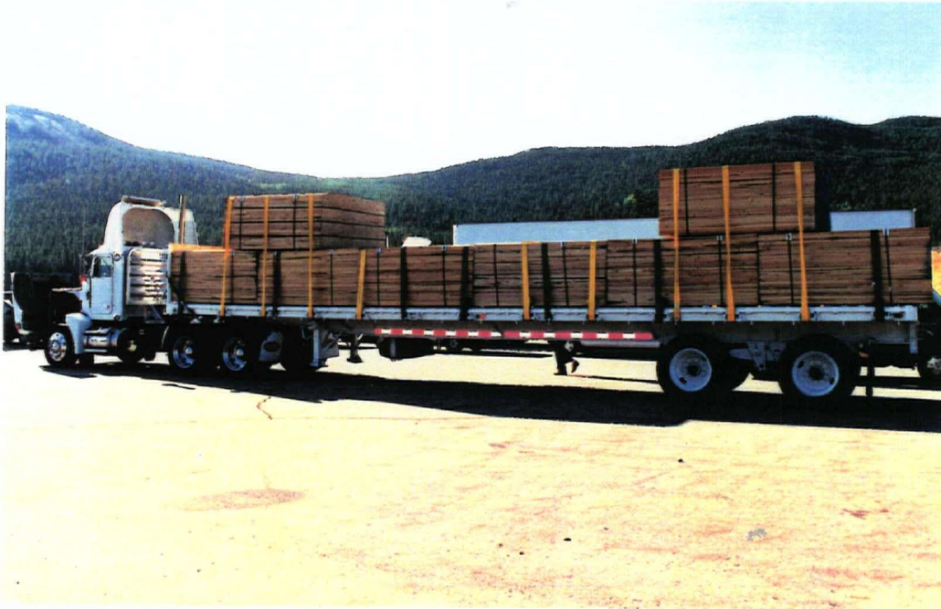
Figure 3.8 Load Configuration on the Trailer
