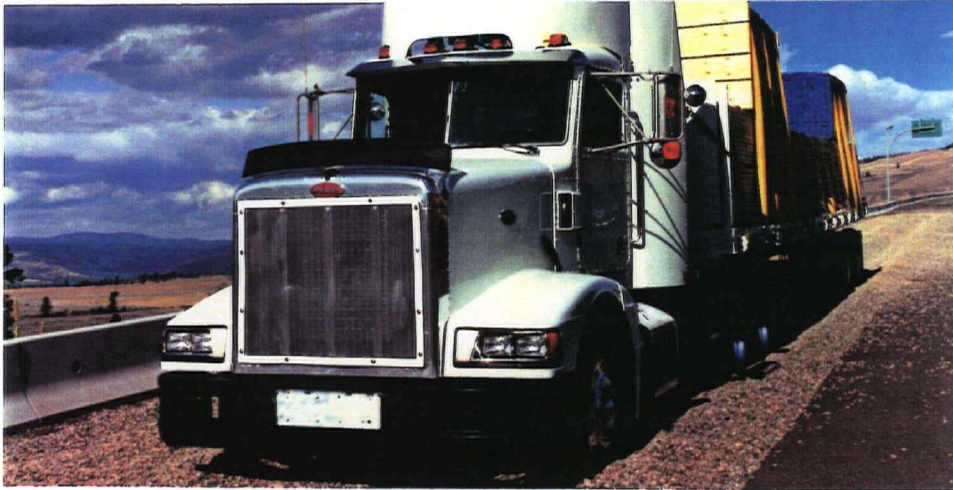
Figure 4.3 Runaway Truck Embedded in an Arrestor Bed
