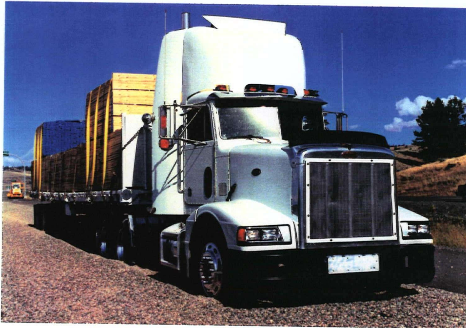
Figure 3.18 Final Resting Position of Truck in Arrestor Bed
