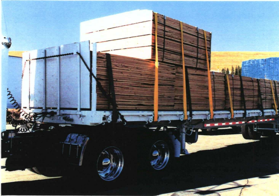
Figure 3.9 Front Stakes to Prevent Load Shift into the Cab
