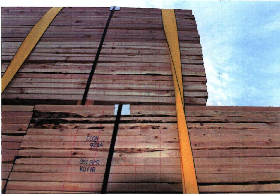
Figure 3.13 Chalk Lines to Identify Load Shift
