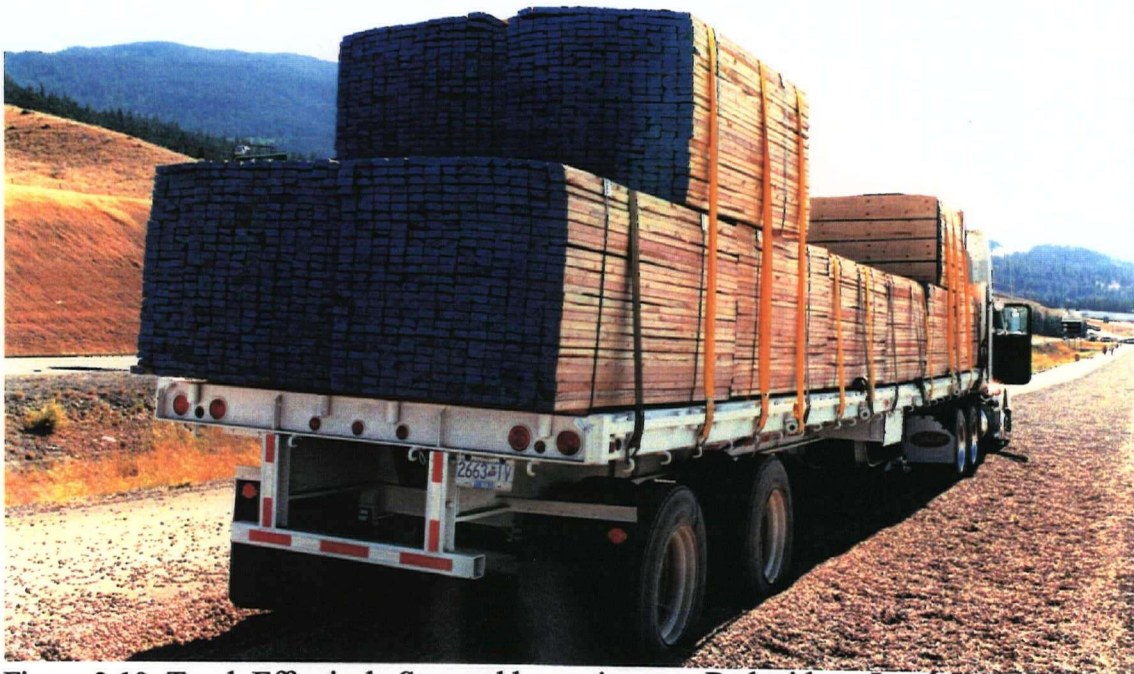
Figure 3.19 Truck Effectively Stopped by an Arrestor Bed with no Load Shift
