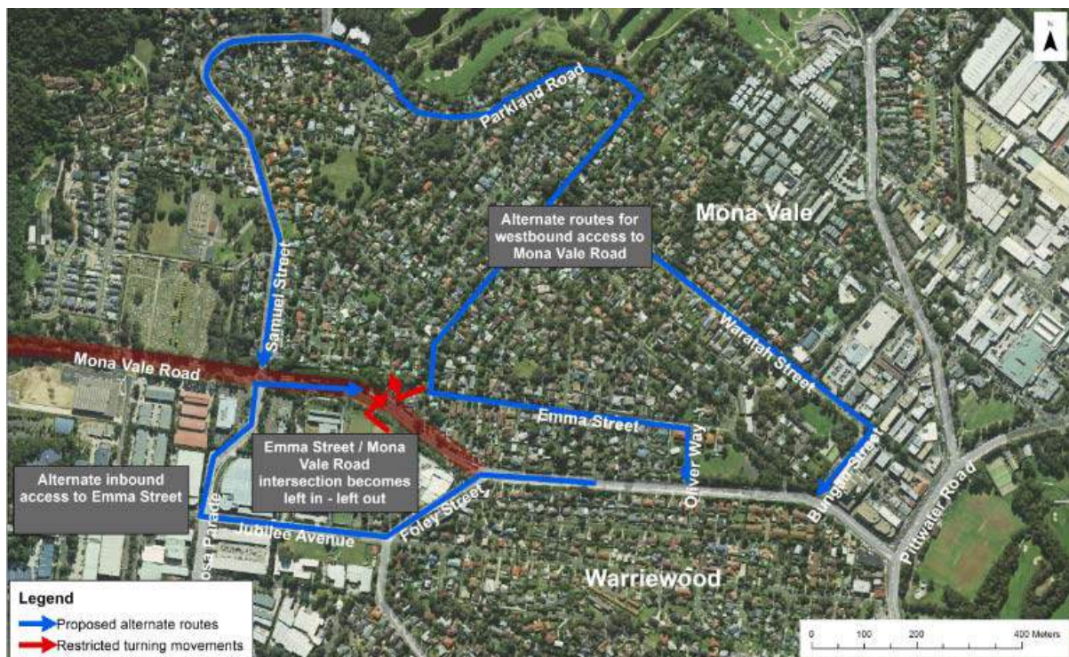
Figure 2-2 Alternate routes (identified in the REF) with Emma street operating as left-in / left-out
